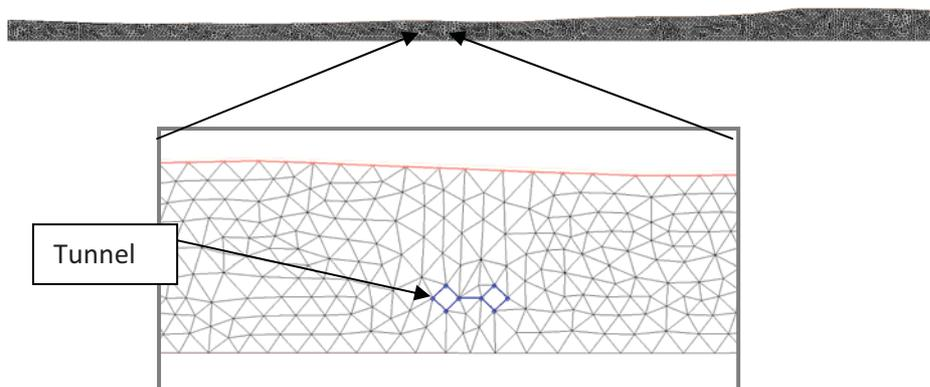
Figure 5-5 FEFLOW model mesh for the Model between Fairfield and Yeronga
