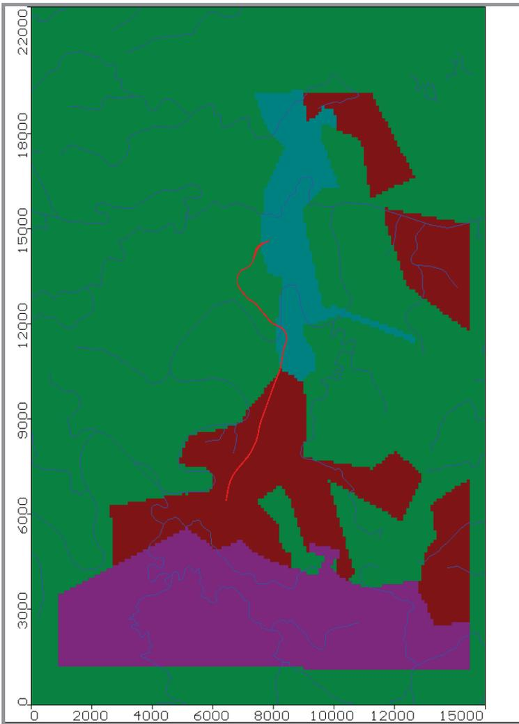
Figure 5-2 Geological Units included in the Model
