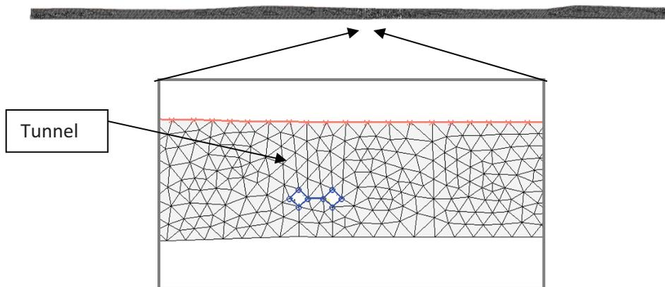
Figure 5-4 FEFLOW model mesh for the Model near Albert St Station
