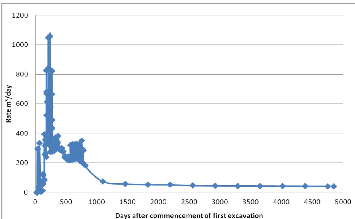
**Figure 5-9 Modelled tunnel drain inflows**
