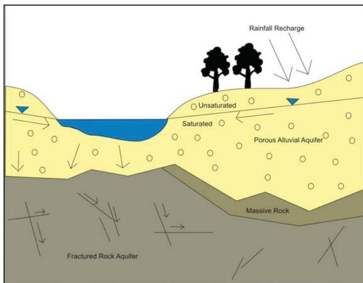
**Figure 3-2 Model 2 Alluvial Aquifer**
