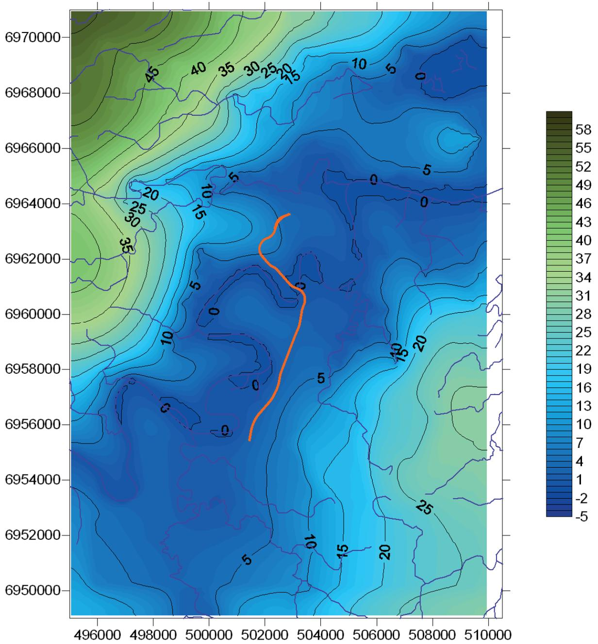
Figure 5-8 Simulated Potentiometric Surface (m AHD)
