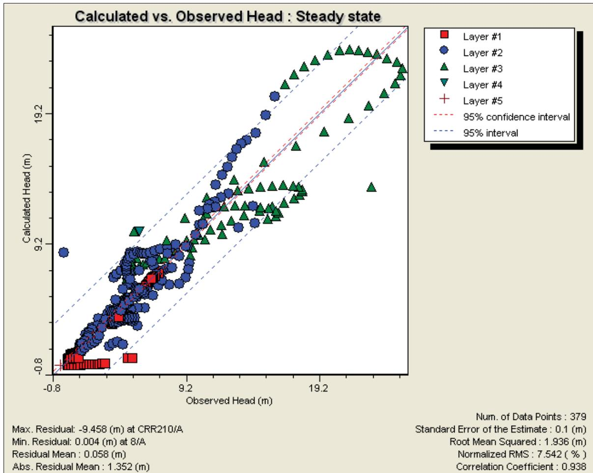
**Figure 5-6 Simulated vs Target Heads**
