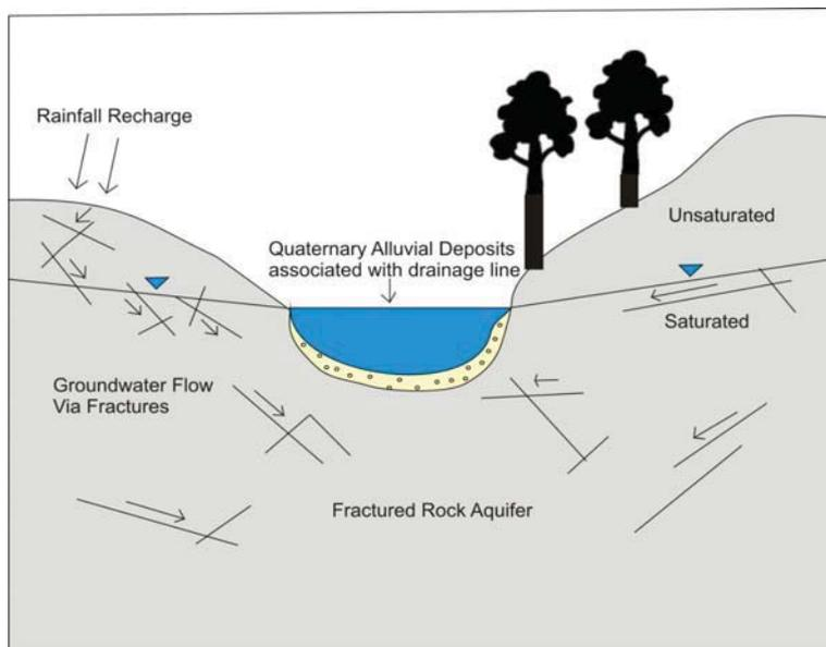
**Figure 3-1 Model 1 Fractured Rock Aquifer**
